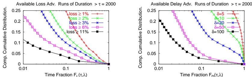
**Fig. 3. Available Loss and Delay Advantage:** CCDF of Time Fractions  $F_L(\tau, \lambda)$ ,  $F_D(\tau, \delta)$  over all SD pairs. Time fraction in which loss advantage exceeds threshold for  $\tau = 2000$ s. Left: loss. Right: delay.
