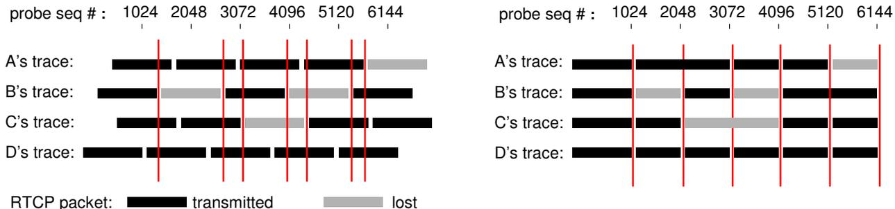
Fig. 3. ALIGNMENT. Without alignment (left), sequence number boundaries of RTP packets are not coordinated amongst receivers, and hence RTP packet loss gives rise to complex patterns of overlap (as delineated by vertical lines). Alignment of packet boundaries (right) promotes overlap in the presence of RTP loss.
